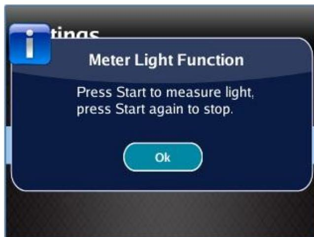
Then press CENTRAL BUTTON to answer OK to confirm light measurement mode and press S1 or S2 button to start the evaluation:
