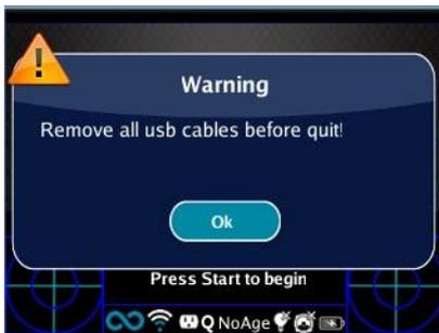
When the device is connected to a computer via USB port the turning off is prevented. When you try to switch off the 2WIN a warning will advise you to remove usb cable.
