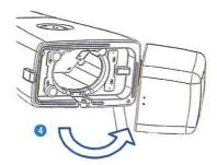
5 - Insert the 2WIN in the device compartment
