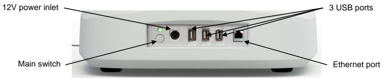
Fig. 2 – Detail of connectors side
