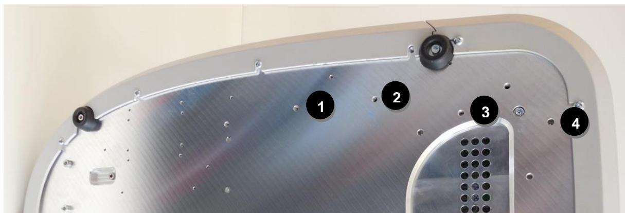
Fig. 12 – Instrument bottom with holes for tablet support
