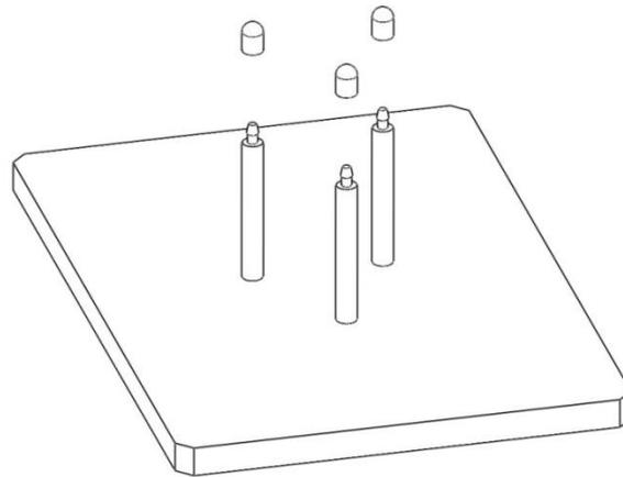
**Figure8-5: Detector Pins and Caps**
