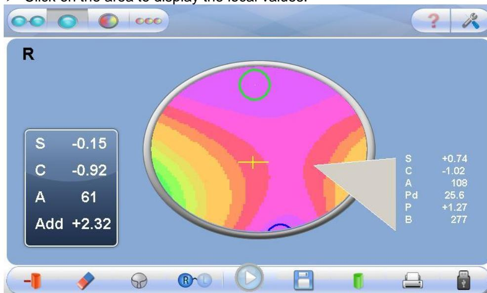
Figure 6-2: Measurement readout for a single point
