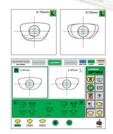
Operators can choose between optical and geometric-centered layouts.
