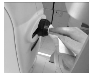
Figure 69 – Clean the lens
