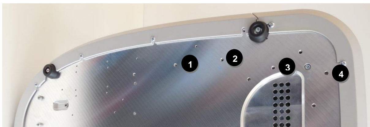
Fig. 7 – Instrument bottom with holes for tablet and joystick supports
