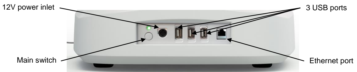
Fig. 2 – Detail of connectors side
