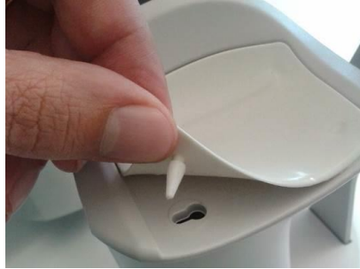
Fig. 41 - Removal of the chin rest silicon pad
