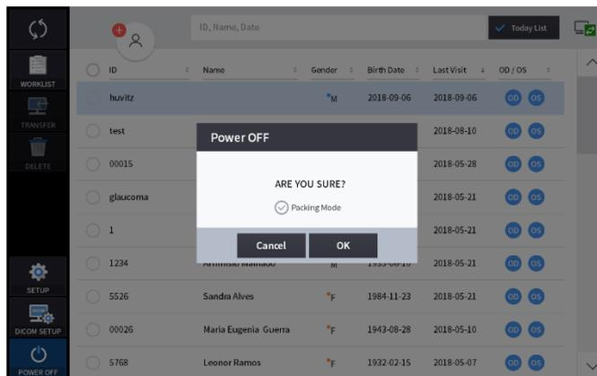
(5) Checking the Packing Mode will move Chinrest and the body of HOCT to the lowest position before Power off (This is for packaging).
