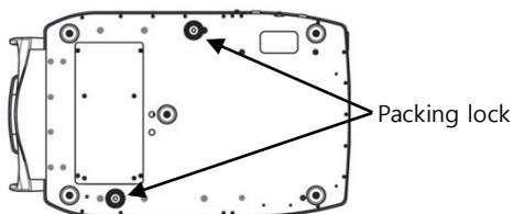
3. Unscrew the user lock lever on the body.
