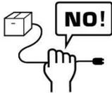
Pull out the power cable with holding the plug, not the cord.
