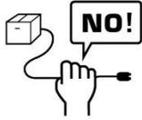
Pull out the power cable with holding the plug, not the cord.
